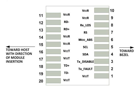
Host PCB SFP Pad Assignment Top View
